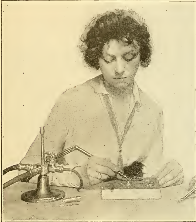
FIG. 91.—Manufacturing Jewelers' and Dentists' Welding Outfit.
